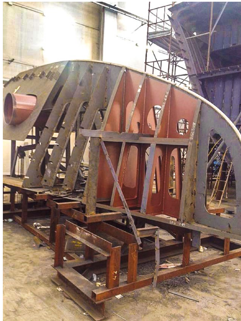
Above, Step by step direct overall control since yacht inception right from the first steel sheet to completion at the Darsena dei Navicelli in Pisa is one of the main features which makes Codecasa stand out. The picture shows the bow end of the C122 being built. The rendering right, Immersed exhausts have been an important evolution for Codecasa. Fine tuning of this aspect was possible thanks to detailed project design work and also in the perfect shaping of the buds.
